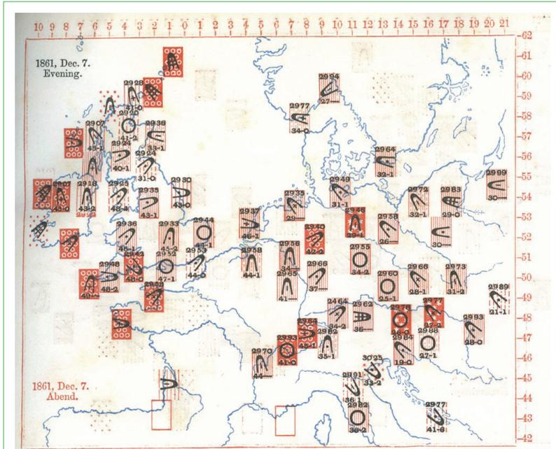
FIGURE 3 Galton's multivariate glyph map of wind direction, strength, cloud cover and rain for one of 93 time points: 7 December 1861, 9pm. The U-shaped icons open in the direction of the wind and are filled in relation to its strength. Stippled and hatched backgrounds range from clear to degrees of cloud, rain and snow. From *Meteorographica*;<sup>10</sup> image courtesy of Stephen Stigler, private collection.
