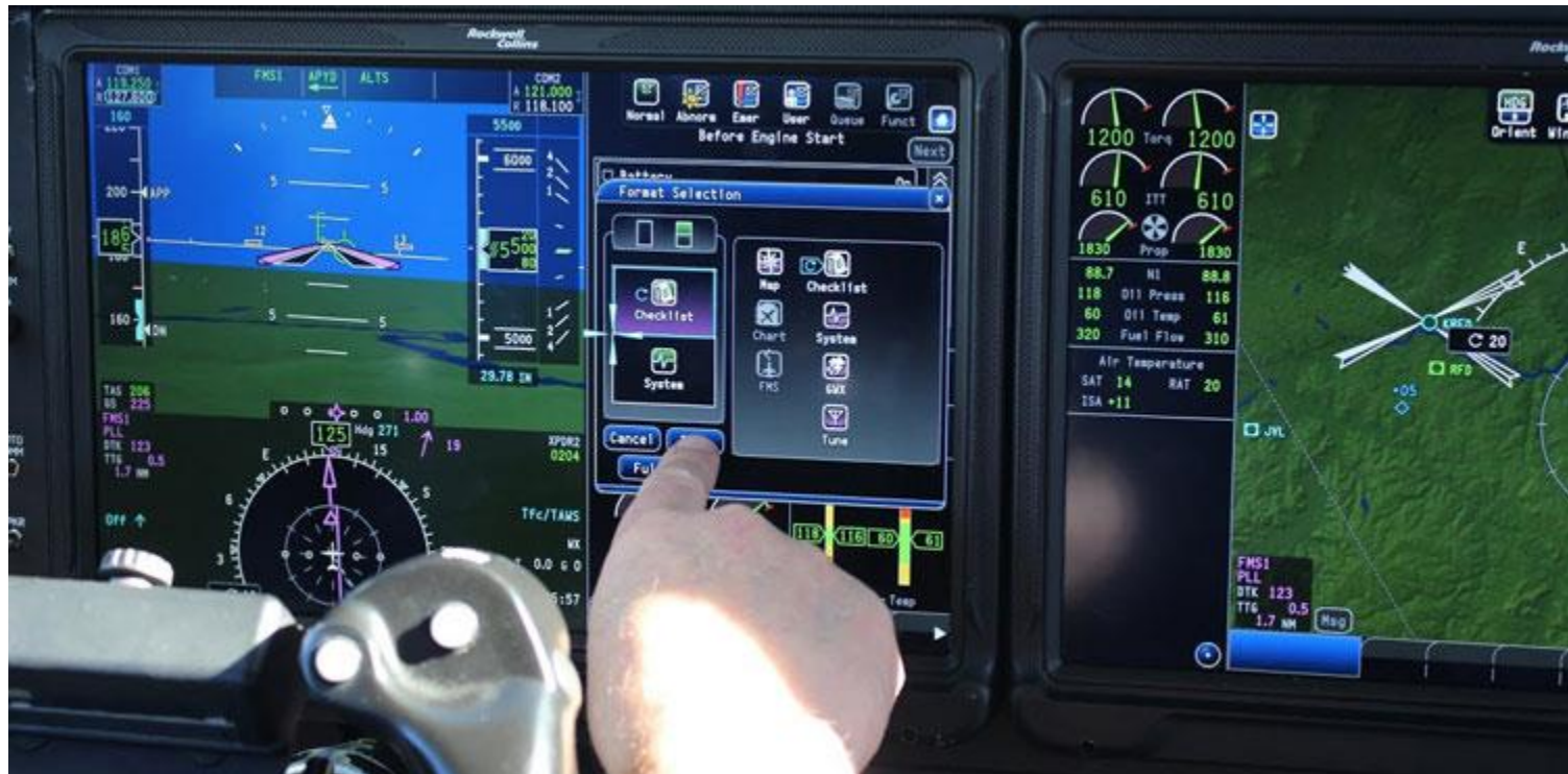
Rockwell-Collins Air King control panel
